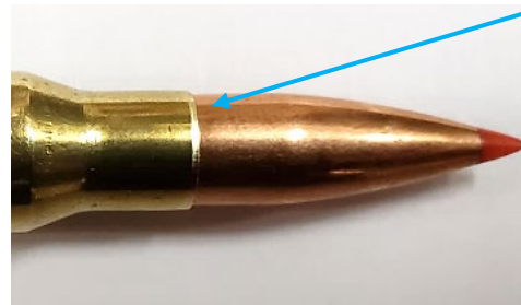
Excessive crimp may show up as a "bright ring" at the top edge of the case neck
