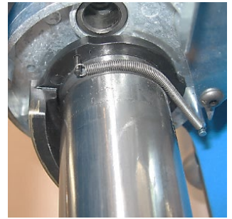
Reinstall Index Ring Spring
