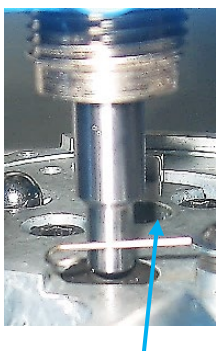
Alignment Fixture entering the Primer Hole
