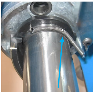
Carefully remove Indexer Return Spring from the two pins
