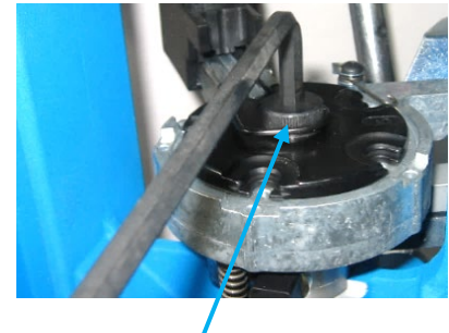
Remove Bolt and replace Shellplate
