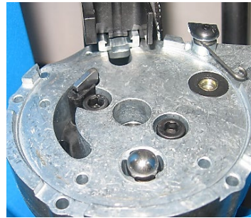
Reinstall Index Pawl and Spring and Index Ball and Spring
