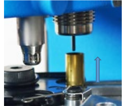
Station 1-Case Inserted into Size De-prime Die—down stroke
