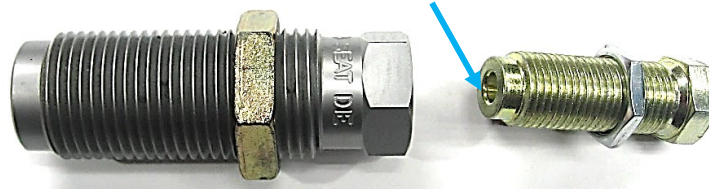
Bullet Contacts Edge of Seating Stem
