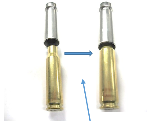
Rifle case neck fits up inside Caliber Specific Powder Funnel to Activate Powder Measure
