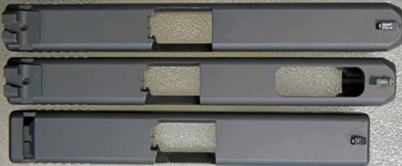
G41 Gen 4 caliber .45ACP slide (top) shown here with G35 Gen4 caliber .40 S&W slide (center) and G21 Gen4 caliber .45 ACP slide (bottom). Note absence of rectangular cutout on the G41 slide and its slightly longer length to accommodate the longer .45 ACP cartridge. Slide thicknesses of both the G41 and G35 slides are 1 inch, while that of the shorter G21 slide is 1.12 inches.
