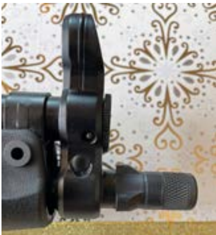
The AP-5 barrel is chrome lined and topped with a tri-lug mount as well as 1/2x28” threads covered with a protector to allow mounting of flash hiders and suppressors.
