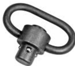
M AGPUL push-button quick-detach sling swivel for 1-1/4" webbing, compatible with QD sling attachment points. Manganese-phosphate finished steel.
