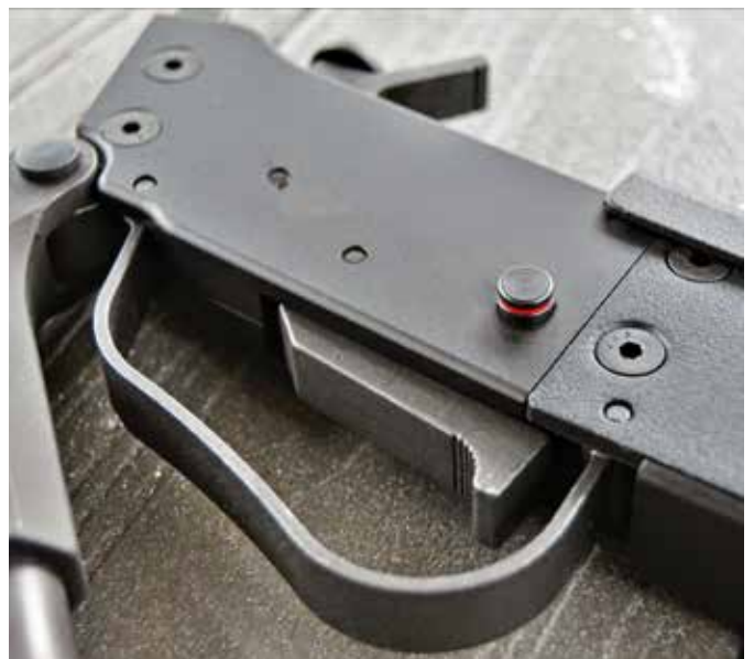
Featuring a squeeze trigger and crossbar safety, this M6 is both the same and different from the original.
