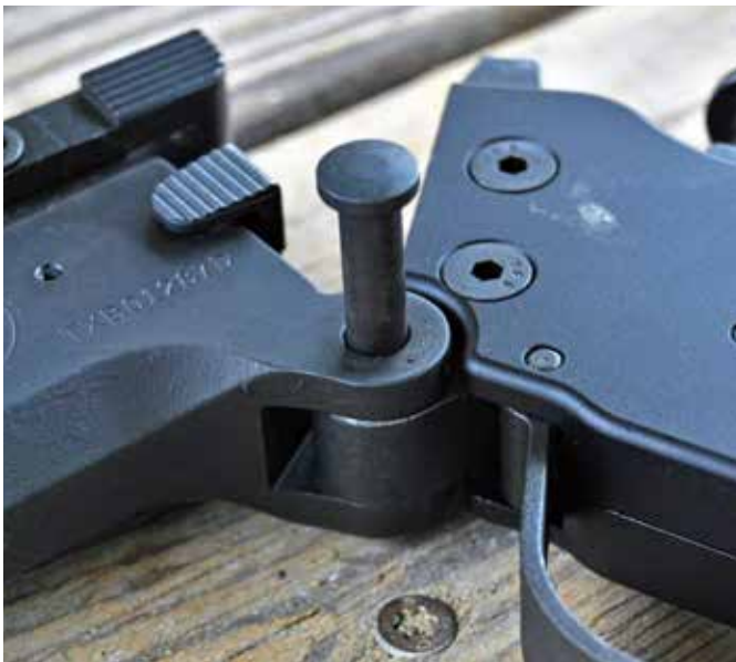
The M6 Takedown's most noticeable improvement is the AR-style takedown pin that is retained in the receiver.
