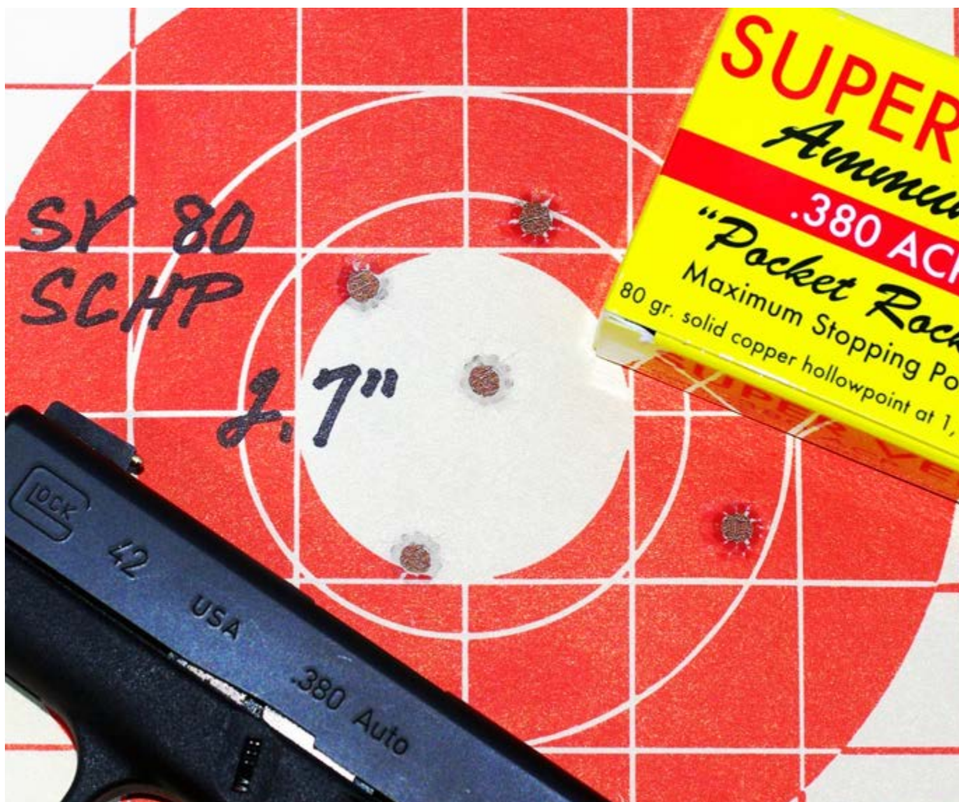
The “perfected” GLOCK 42 put five rounds of Super Vel 80-grain Solid Copper HP into 2.7”, well-regulated for windage and elevation, at 50 feet from the bench.
