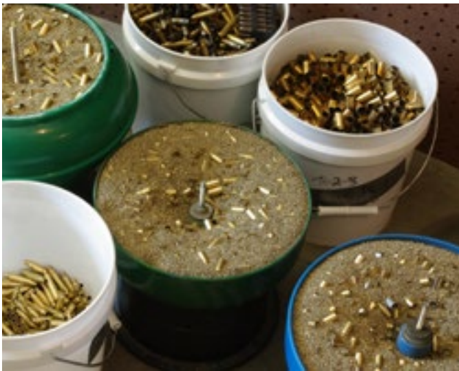
Range brass must be cleaned. Here is brass in corncob media in vibrating brass cleaners. Buckets of brass wait their turn.
