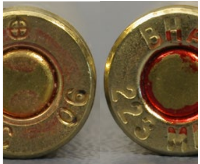
Notice the crimped primer pocket on the left.
