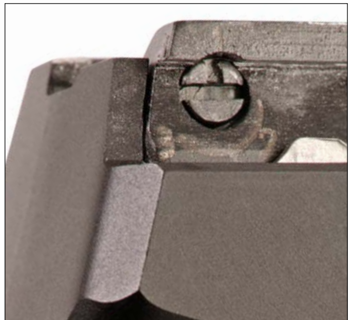
Top left of the frame features a three-position rotary switch (see inset at right ) controlling the magazine disconnector and the grip safety.
