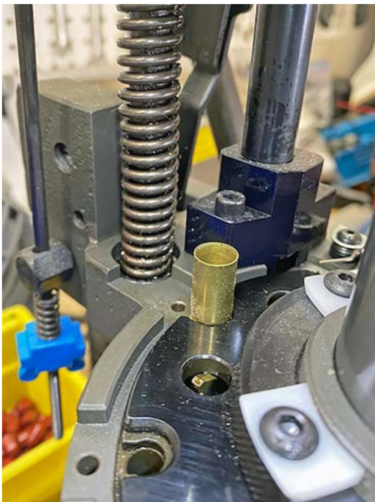
"I have the locator buttons removed from the powder station and the station immediately after it. I'll individually insert the case under the powder die for every drop, and once the powder is in the case, I'll immediately remove it at the next station for measurement."
