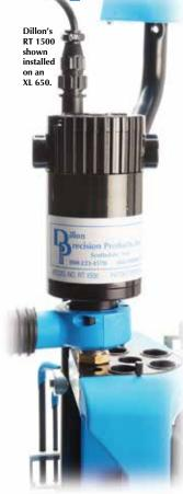
he RT 1500 is used just like a standard size die. The big difference is that while you are pushing the case into the die to size it, an electric motor driving a carbide cutter at 4500 RPM is trimming the case to length. Chips are drawn off through a vacuum manifold that clamps to the outside of the special size/ trim die. (Vacuum cleaner and hose not included.) The RT 1500 is equipped with a
