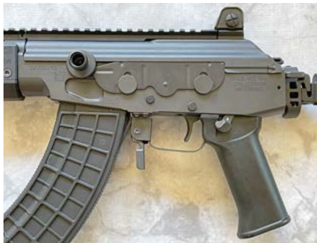
Galil ACE left side view. Note charging handle, FNC style side dust cover mechanism, original grip and thumb safety. Magazine is an X-Tech.
